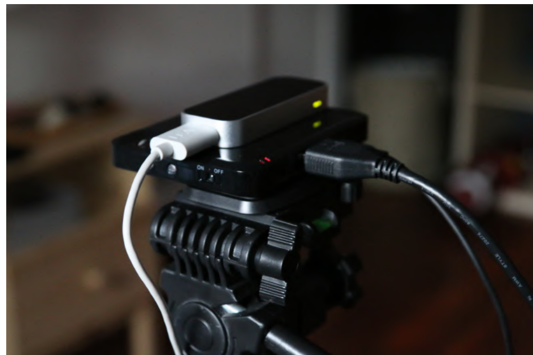
Mounted Pico Projector & Motion Sensor
